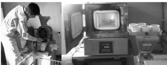
Fig. 3: Crushing of the waste, Incineration of waste of Lab scale
