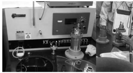
Fig. 4: Determining calorific value of the waste.
