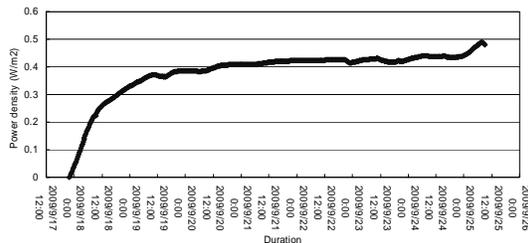
Fig. 3: Variation of power density with duration
