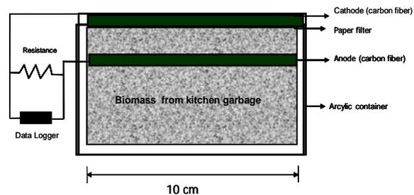
Fig. 1: Schematic diagram of MFC in Laboratory
