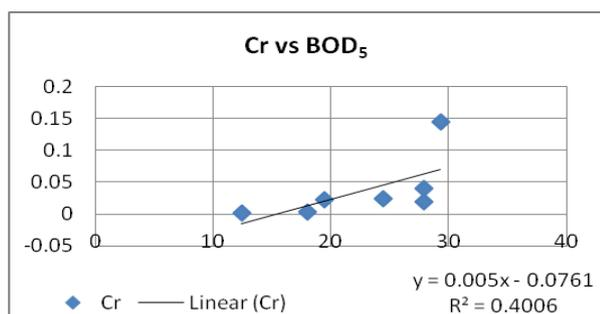
Fig. 5. Graphical presentation of the correlation between Cr and BOD<sub>5</sub>
