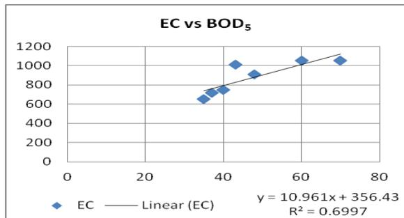
Fig. 3. Graphical presentation of the correlation between EC and BOD<sub>5</sub>
