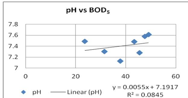
Fig. 6. Graphical presentation of the correlation between pH and BOD<sub>5</sub>
