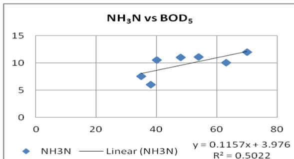
Fig. 4. Graphical presentation of the correlation between NH<sub>3</sub>-N and BOD<sub>5</sub>
