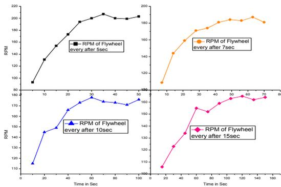
Fig. 5. Merged experimentally obtained rpm w.r.t. time of flywheel
