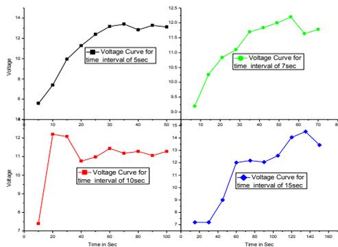
Fig. 6. Merged experimentally obtained voltage w.r.t. time of generator
