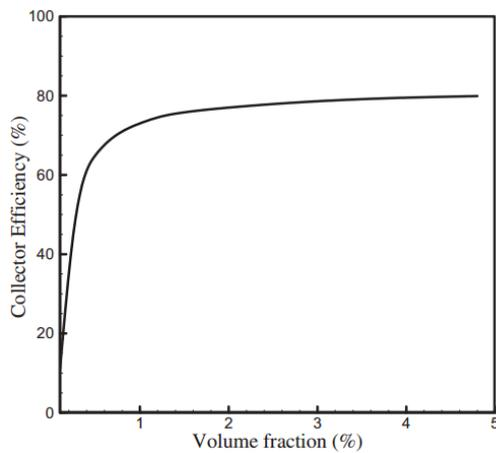
Fig. 3: DASC efficiency vs. volume fraction.
