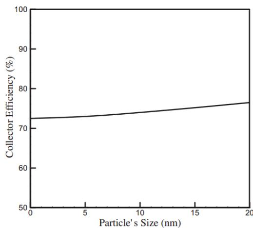
Fig. 4: DASC efficiency vs. particle size at 0.8% volume fraction.
