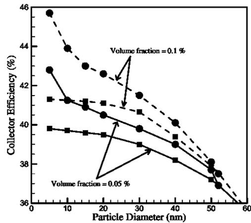
Fig. 5. Collector efficiency vs. particle diameter for silver particle in micro scale direct absorption solar collector.
