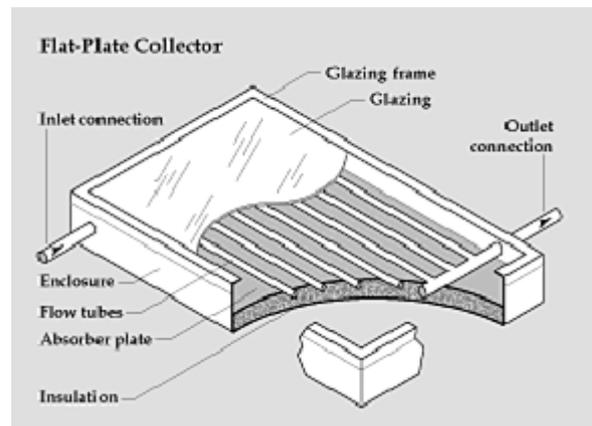
Fig. 1. Schematic diagram of a flat plate solar collector.
